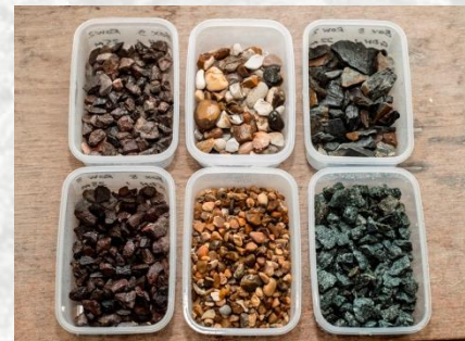
Photograph showing several washed aggregate samples from quarries across the UK and the Republic of Ireland.
