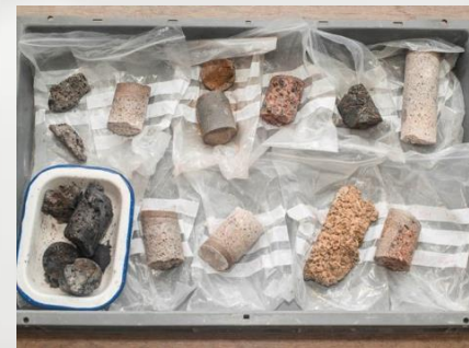
Concrete core and chisel samples are received from the surveyor for a Stage 1 screening test. Samples are laid out in numerical order, measured, weighed and washed before analysis.
