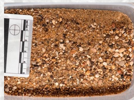
Photograph showing an example of well-graded and fine-grained river sand aggregate.
