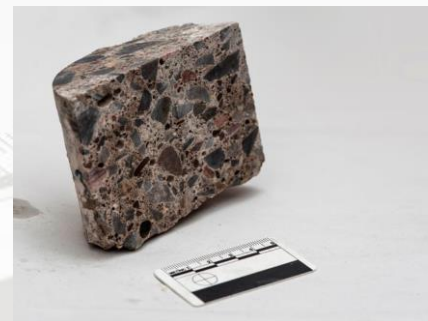
Photo showing a sliced section of concrete to be prepared for sectioning and petrographic analysis.
