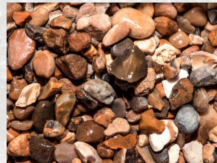
Photograph showing an example of a coarse aggregate consisting primarily of a chert gravel.
